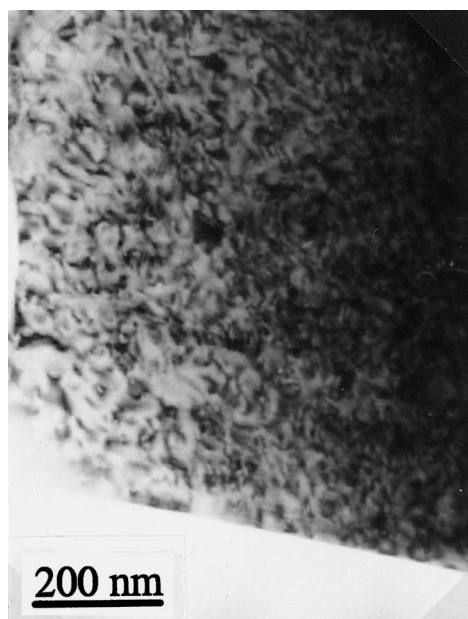
Fig. 2. TEM image of neutron-irradiated \text{Al}_2\text{O}_3 ( 1.7 \times 10^{26} \text{ m}^{-2} , 815 K) ( E > 0.1 \text{ MeV} ).
